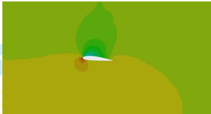
Gambar 32. Distribusi Tekanan Variasi Front Sweep Hydrofoil (Sumber : Data diolah, 2025)
